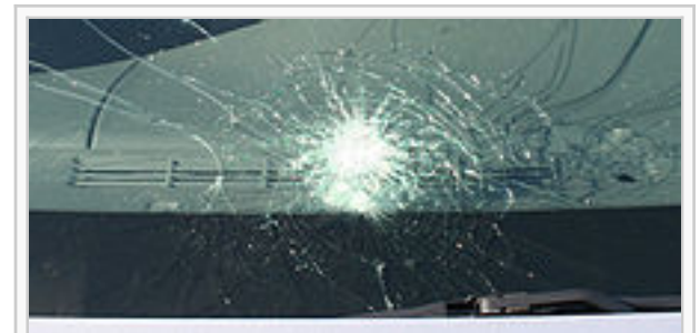
Automobile windshield with "spider web" cracking typical of laminated safety glass.
